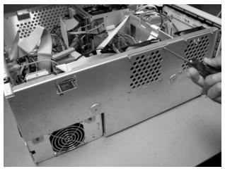
Figure 4-34. Removing the Fan
