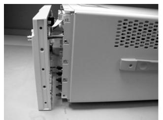
Figure 4-33. Slide Front Panel Away From Mainframe
