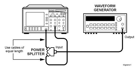
Figure 2-15. Trigger Sensitivity Equipment Setup
