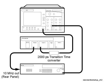
Figure 3-1. Timebase Adjustment Setup
