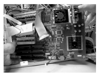
Figure 4-42. Pull the Motherboard out the Right Side
