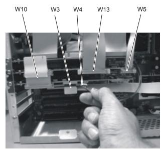
Figure 4-47. W3, W4, W5, W10, and W13 Cables
