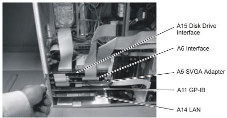
Figure 4-36. Removing the Circuit Boards from the Motherboard
