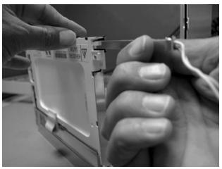
Figure 4-20. Removing the Backlight
