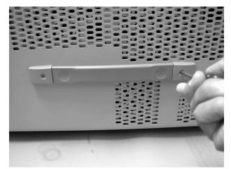
Figure 4-4. Removing the Side Handles
