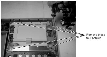
Figure 4-16. Removing the Display Screws
