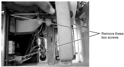
Figure 4-63. Disconnecting Screws from A6 Board
