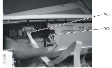
Figure 4-10. Removing the W5 and W6 Ribbon Cables
