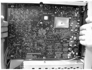
Figure 4-50. Sliding the Board to the Right
