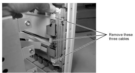
Figure 4-29. Removing the Cables from the Inverter Board
