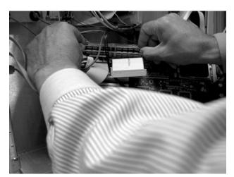
Figure 4-43. Removing the RAM
