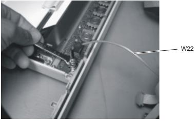
Figure 4-13. Removing the Front Panel Trigger Cable
