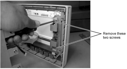
Figure 4-30. Removing the Keyboard Panel Screws
