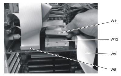
Figure 4-46. W8, W9, W11, and W12 Cables
