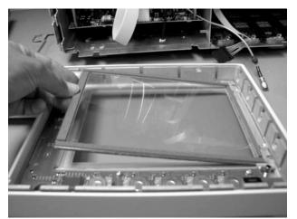
Figure 4-22. Lifting out the Touch Screen
