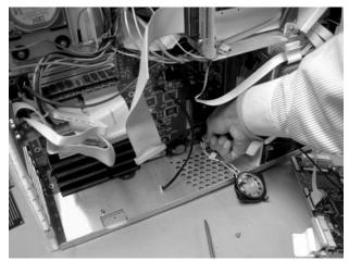
Figure 4-39. Disconnecting the Speaker Cable
