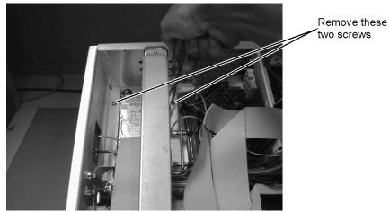
Figure 4-59. Removing the Screws on Top of the Hard Drive
