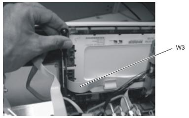
Figure 4-11. Disconnecting the W3 Mylar Flex Cable
