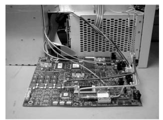
Figure 4-53. Removing the A13 Acquisition Board
