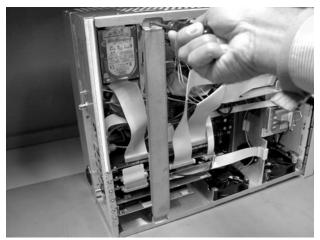
Figure 4-35. Removing the Bar (86100A only)
