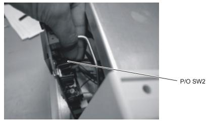
Figure 4-52. Removing the SW2 Cable from P19 Connector
