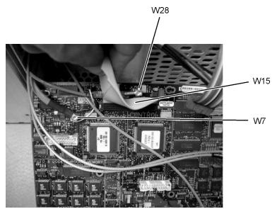
Figure 4-54. W28, W7, and W15 Cables from the A13 Acquisition Board
