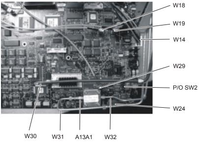
Figure 4-55. Cables from the A13 Acquisition Board (option 001)
