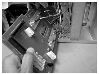
Figure 4-66. Pulling Out the A6 Distribution Assembly Board
