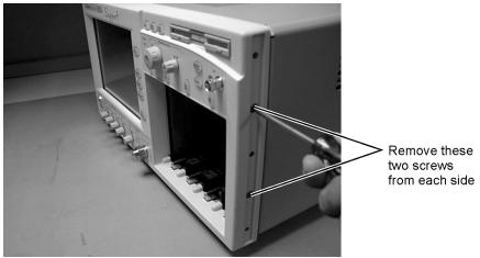
Figure 4-7. Removing the Front Panel Screws
