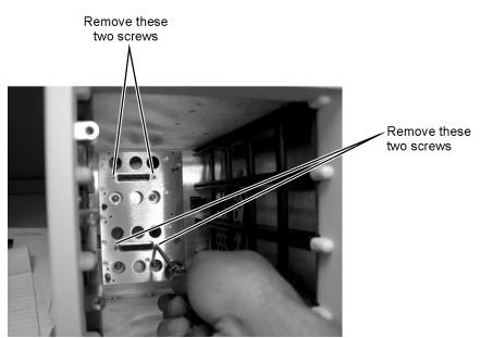
Figure 4-65. Removing Screws from Connectors in Module Drawer
