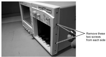
Figure 4-27. Removing the Front Panel Screws
