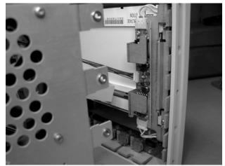
Figure 4-28. Accessing the Inverter Board
