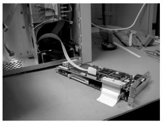
Figure 4-37. Removing the A5 and A6 Boards
