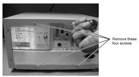
Figure 4-3. Removing Screws from Back of Mainframe
