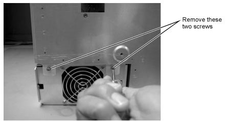
Figure 4-58. Removing the Screws Securing the Power Supply
