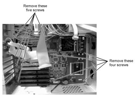
Figure 4-40. Removing the Screws from the Motherboard
