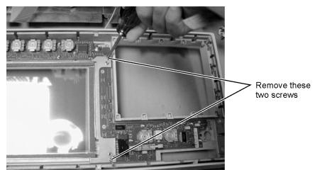
Figure 4-21. Removing the Touch Screen Screws
