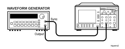
Figure 2-9. Time Interval Accuracy Setup from 20 ns/div to 20  $\mu s/div$
