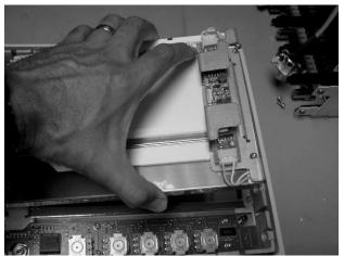
Figure 4-17. Removing the Display
