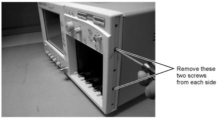
Figure 4-32. Remove the Front Panel Screws
