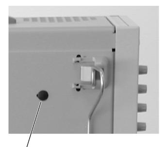
Hole Plug Figure 3-3. Hole Plug Location
