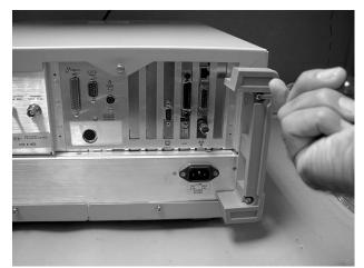
Figure 4-2. Removing the Rubber Feet
