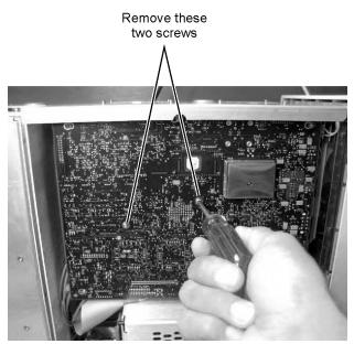
Figure 4-49. Removing the A13 Acquisition Board Screws
