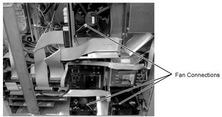
Figure 4-61. Fan Connections
