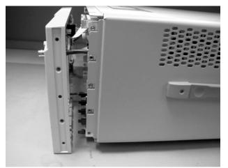
Figure 4-8. Sliding Front Panel Away From Mainframe
