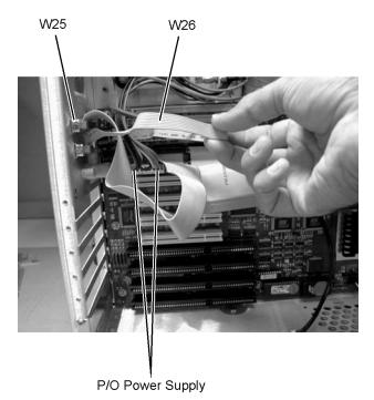
Figure 4-44. W25, W26, and Power Supply Cables
