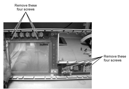
Figure 4-25. Removing the Keyboard Panel Screws
