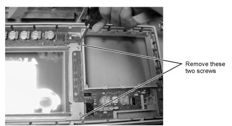
Figure 4-24. Removing the Touch Screen Screws
