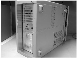
Figure 4-5. Sliding Cover off Mainframe
