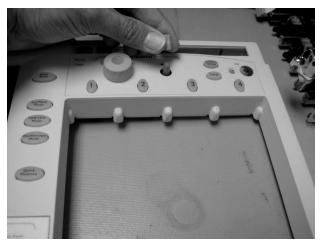
Figure 4-23. Removing the Knobs
