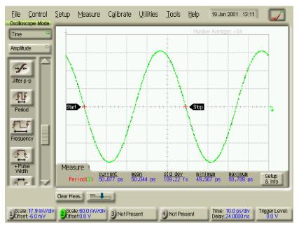
Figure 2-5. Setting Period for Measuring Time Interval Accuracy
