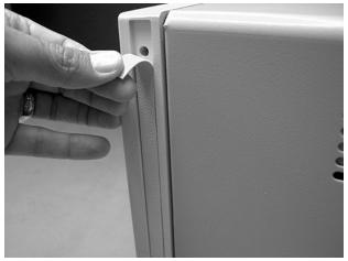
Figure 4-6. Removing the Trim Strips
