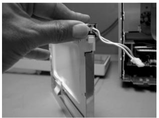
Figure 4-19. Release the Backlight Tab
