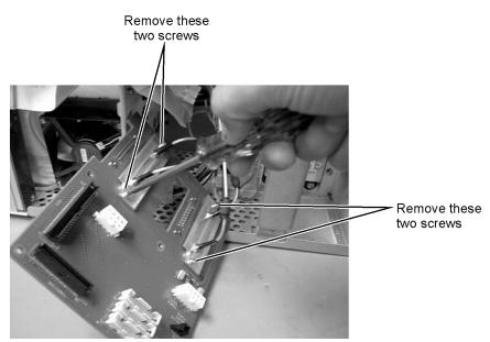
Figure 4-67. Removing the Screws from the A6 Bracket
