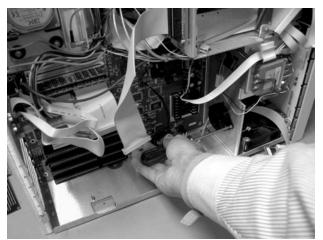
Figure 4-38. Removing the Speaker Screw
